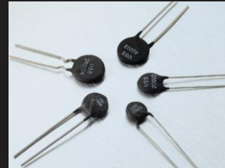
Thermistor: Temperature changes resistance
