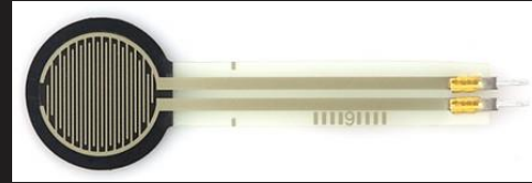
Force Resistor: Pressure changes resistance
