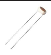
Photoresistor: Light changes resistance
