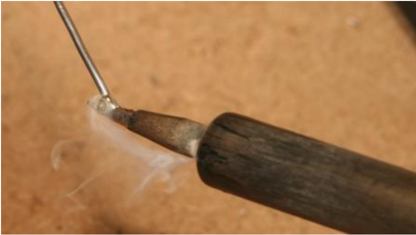
Apply Solder to Soldering Iron Tip
