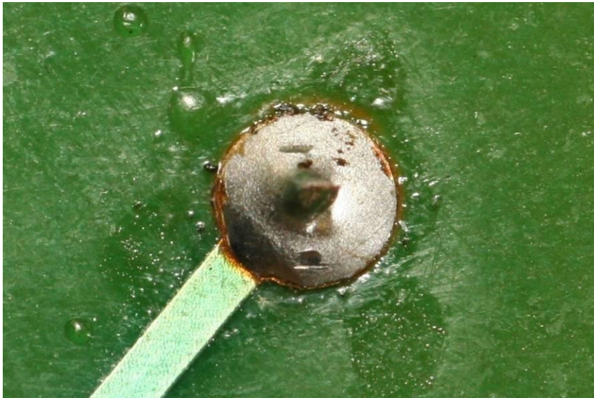
Cold Solder Joint
