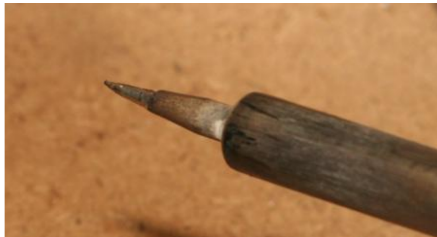
Properly Tinned Soldering Iron Tip
